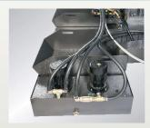
■ High pressure pump unit provides sufficient pressure for the coolant system to cool off the heat generated from tools and workpiece machining.
