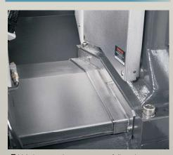
Y Axis protection cover uses full enclosure type to prevent cutting chips from entering Y Axis drive system that affects the system precision.
