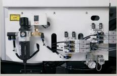
■ The Pneumatic Unit has pressure sensor, the system will generate alarm message when the pressure is insufficient to ensure normal operations of the machine.
