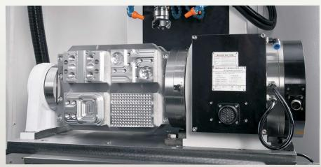
■ The 4th Axis provides special tailstock support design for the fixture to expand the machining space between fixture and workpiece.
