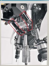
■ Before the tool change, the tool holder chip wash down system can wash clean the chips attached to the tool to ensure that the tool is closely fit after tool change.
