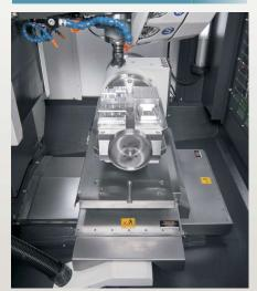
Optimum design of operation space enables easy collection and cleaning of cutting chips.
