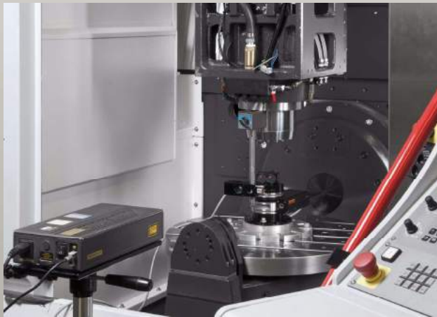
■ Worktable Center Calibration w/ Heidenhain TS740. High Precision Touch Probe & Standard Calibration Ball with Heidenhain Measurement Software can detect error value of the worktable and compensate to ensure Worktable Precision.
